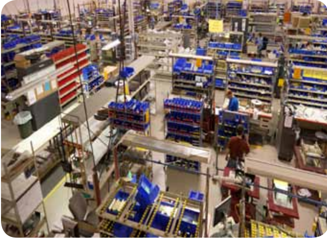
All of DeCrane's assembly cells are arranged based on the seat model and customer specification.
