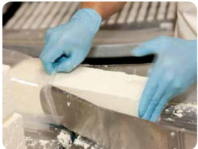
*The bricks of feta cheese are placed into plastic pouches for vacuum sealing.*
