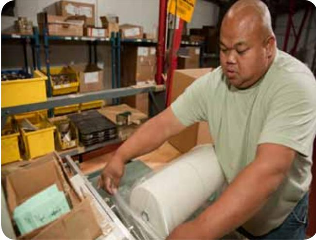
*Sing Sayarath vacuum packs filters to prevent the sensitive media from absorbing water from the air during shipping, an critical step in serving international customers.*
