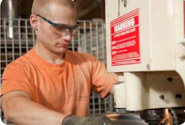
*Mark Bilhorn operates the hole-punch machine to prepare canister lids for assembly.*
