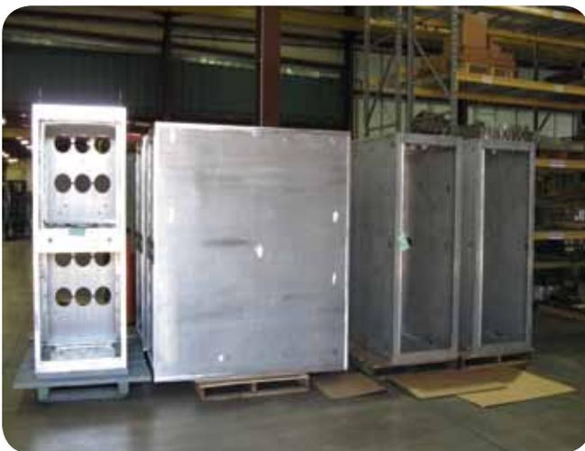
*Cabinets in-process in the staging area prior to chemical coating process.*
