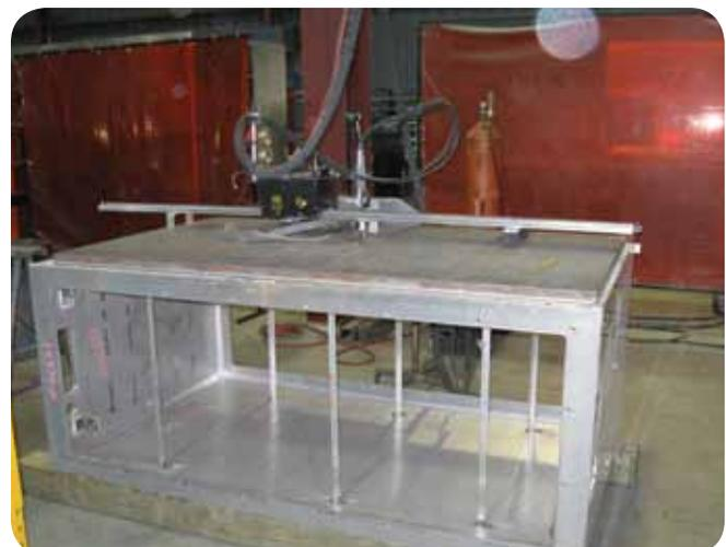
*The semi-automatic welder makes a 6 foot weld on outside edge of cabinet.*
