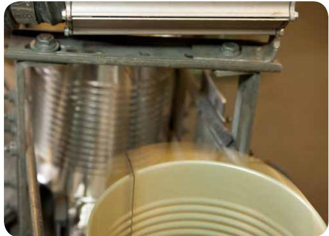
*Blowers are used to blow debris from cans as they move through the automated assembly line.*
