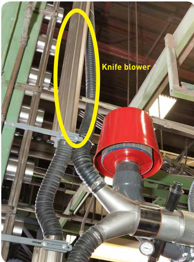
Cans move on a conveyor as air from a knife blower cools the weld. Blowers provide results equivalent to that of expensive compressed air.
