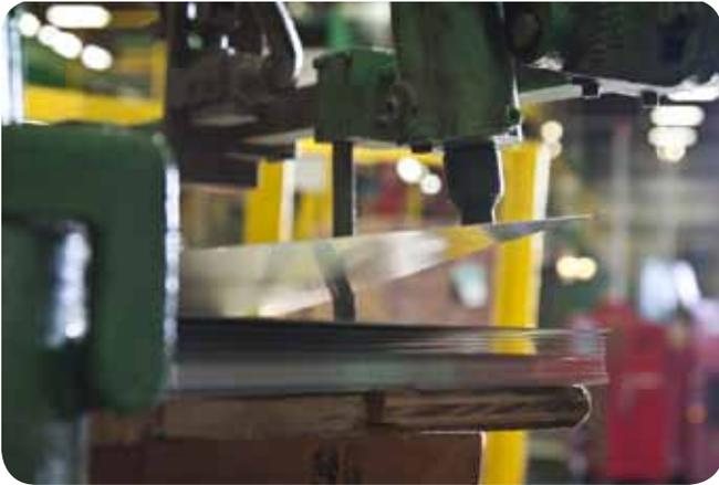
*Blowers are used to separate sheets of metal so that they can be individually cut to the proper size to manufacture cans.*
