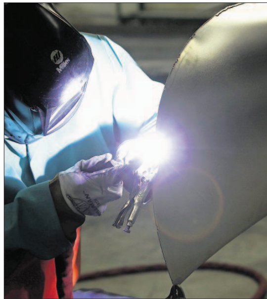
Crafting: Glenn Walton welds a canoe at Osagian Canoes in Lebanon, Mo. The company's aluminum canoes have hull pieces that are welded rather than riveted.
