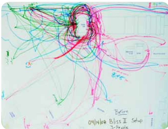
The spaghetti diagram illustrates the steps each of the three employees make when changing the die on the SUV.
