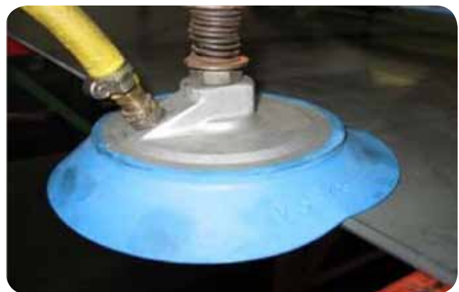
One of the many equipment maintenance initiatives included a new jib crane lift cup.
